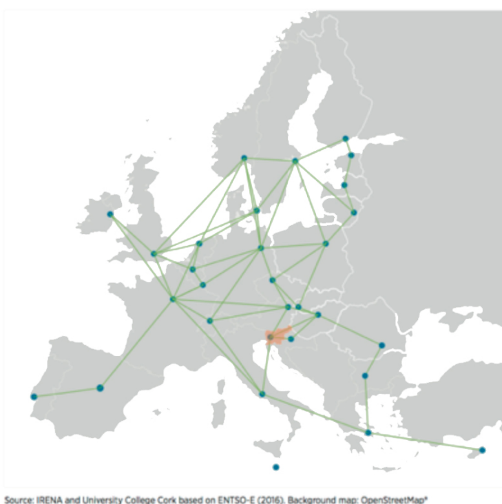
Figure 1 – Interconnections in the 2030 EU power system model 83
